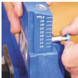
▲ The spring-loaded indexing pin is used alongside the height scale on the side that relates to timber thickness
